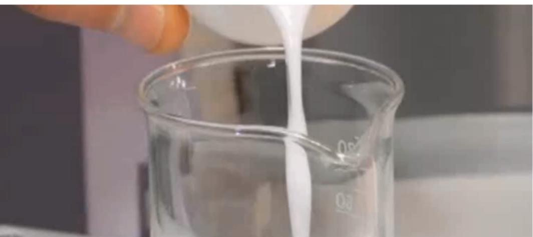
I FLUIDI ELETTROREOLOGICI SONO COSTITUITI DA PARTICELLE POLARIZZABILI DISPERSE (INORGANICHE O ORGANICHE) IN UN FLUIDO NON CONDUTTORE A BASSA VISCOSITÀ (GENERALMENTE OLIO SILICONICO). SONO MATERIALI CHE MODIFICANO LE PROPRIE CARATTERISTICHE REOLOGICHE (E.G. VISCOSITÀ) MEDIANTE L'APPLICAZIONE DI UN CAMPO ELETTRICO CON INTENSITÀ PARI AD ALCUNI  $kV/MM$ , PASSANDO DALLO STATO LIQUIDO ALLO STATO QUASI SOLIDO CON VELOCITÀ DELL'ORDINE DEI MILLISECONDI.
